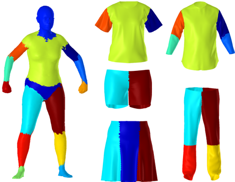
Figure 7: Color-coded body and clothing. The colors show the part correspondences between bodies and clothing. During training, the rigid rotation for each clothing part is the same as the rotation for the corresponding body part. This allows us to transfer a new body pose to the clothing during clothing fitting.
