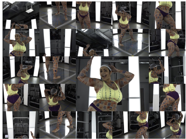
Figure 2: 4D scanner. Our scanning system captures full-body 3D mesh sequences at 60 fps using active stereo. The color image from each of 22 scanning units is shown (see text).
